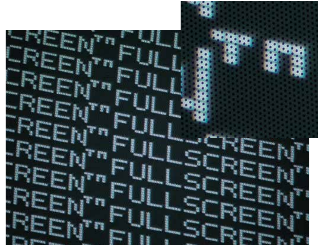
Segment of projected image, VELVET/DIGIGON (test image) Lateral color: negligible – less than 1/4 pixel width Exposure data: Canon EOS 5D Mk II, ZEISS Macro-Planar
