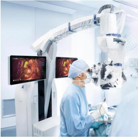
Fluorescence is the property of atoms and molecules, so called fluorophores, to absorb light at a particular wavelength and to subsequently emit light of longer wavelength. Fluorescence microscopy can be based on autofluorescence or the addition of fluorescent dyes.<sup>1,2</sup> Under normal light fluorescent dyes might be invisible. But a surgical microscope with integrated fluorescence technology lights up the dye to visualize tumor tissue or blood vessels during surgery.
